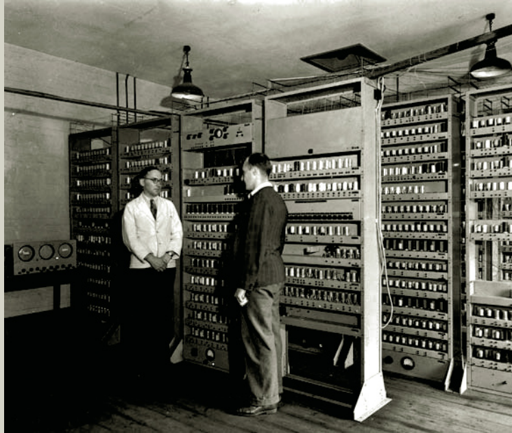
EDSAC (Electronic Delay Storage Automatic Computer)
